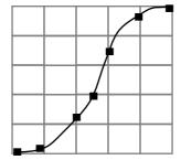
You should enter two level/volume breakpoints at the minimum and maximum levels and several for each place where the vessel has got an arc. You can enter any number of pairs between 2 and 16.
