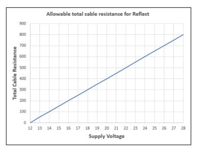
Maximum cable resistance vs supply voltage.
