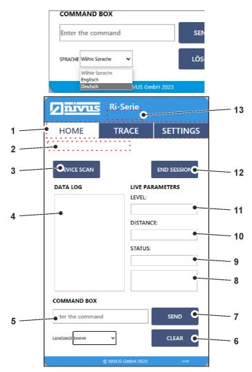
**1. Web Page Selector:** Displays the current NIVUS Ri-Series radar sensor page you are viewing highlighted by a white background.
